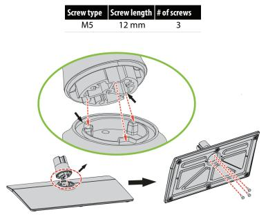
3 Align the stand cover with the column, then secure the cover to the column with one of the provided screws. Make sure that the bottom of the cover is flush against the top of the column.
